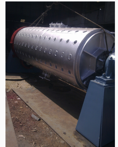
Ball Mill 3000 Ltrs. Capacity
